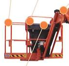
Cylinder boots protect cylinder shafts from debris
